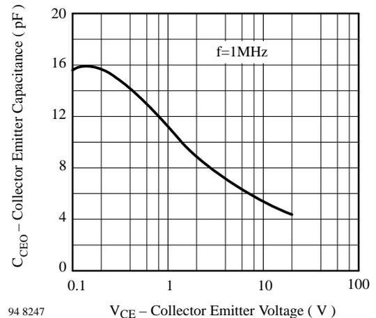
Figure 8. Collector Emitter Capacitance vs. Collector Emitter Voltage
