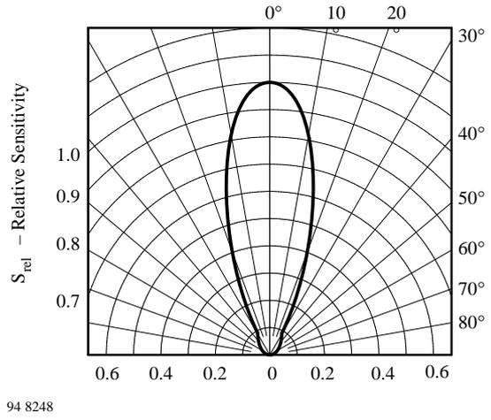
Figure 11. Relative Radiant Sensitivity vs. Angular Displacement
