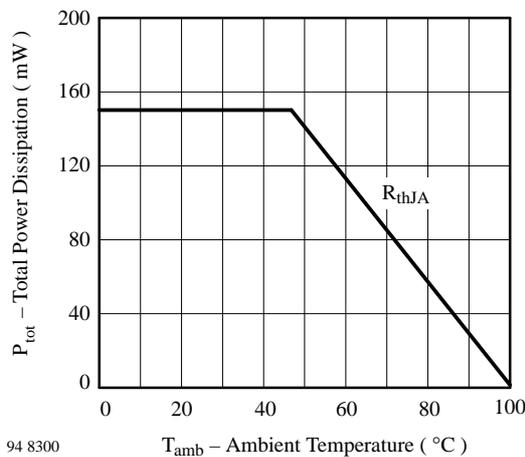
Figure 1. Total Power Dissipation vs. Ambient Temperature
