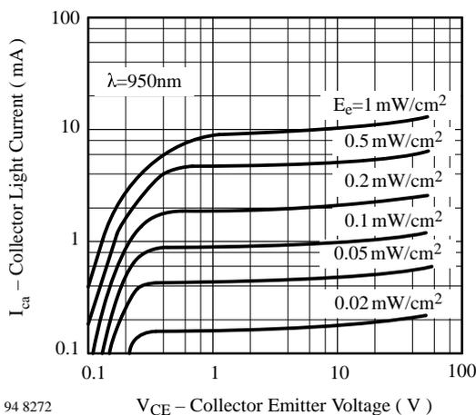
Figure 5. Collector Light Current vs. Collector Emitter Voltage
