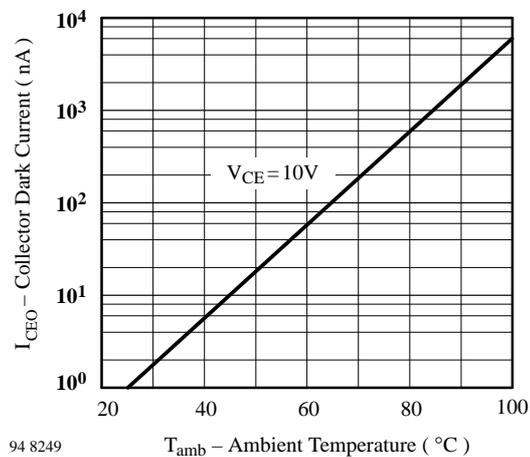
Figure 2. Collector Dark Current vs. Ambient Temperature
