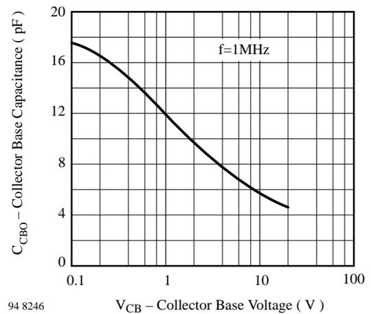
Figure 7. Collector Base Capacitance vs. Collector Base Voltage
