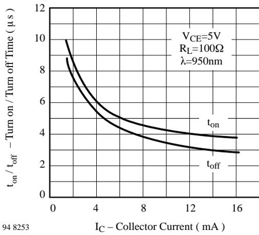
Figure 9. Turn On/Turn Off Time vs. Collector Current
